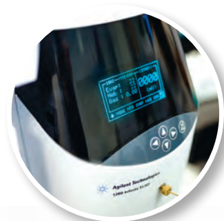
Detecting contaminants such as banned substances using ELSD (Evaporative Light-Scattering Detector)
