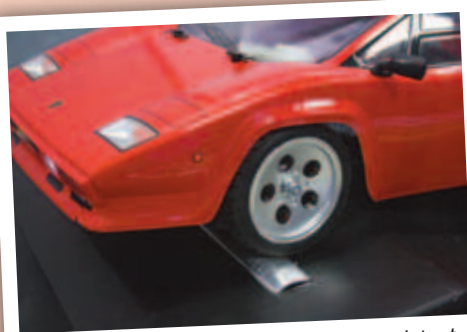
A limit switch serves as the sensor to detect an approaching car
