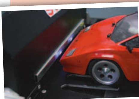
A second limit switch detects that a car has smashed into the barrier
