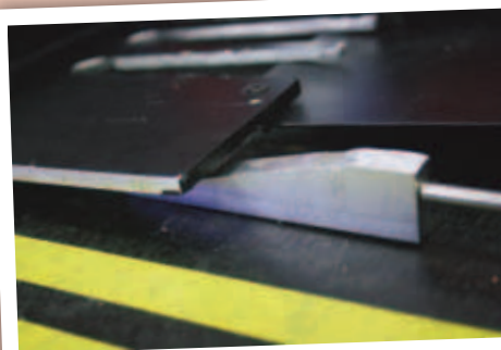
Two water hydraulic cylinders then drive a wedge under the movable ramp, thereby lifting up the car
