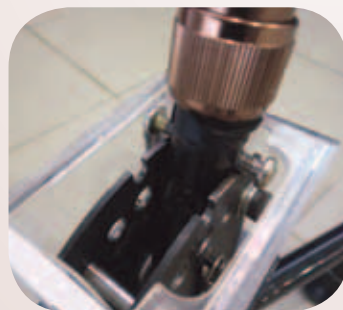
The tilting mechanism at the base of the handle
